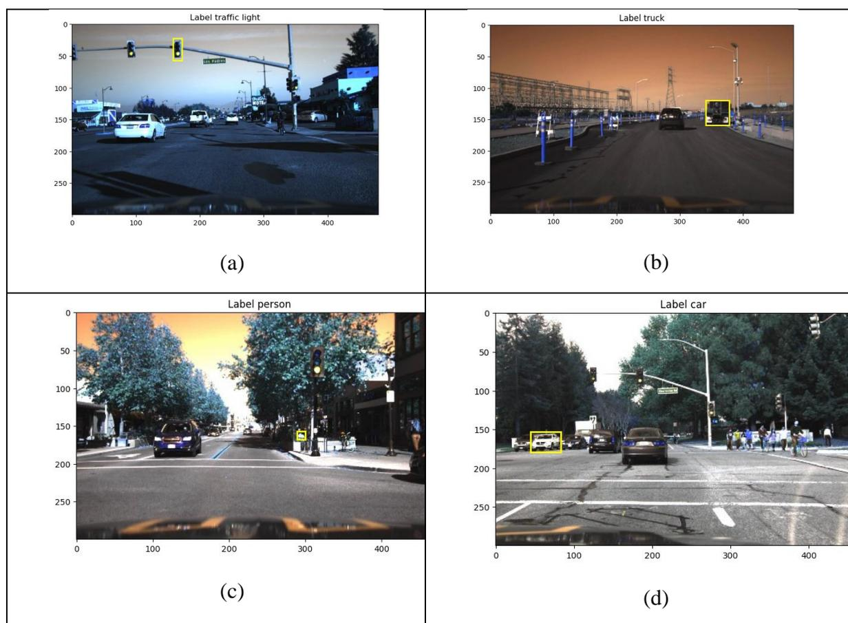
**Figure 5(a).** Traffic light detection, (b) Truck detection, (c) Pedestrian detection, and (d) Car detection output of the proposed HCNN-TMOD method
